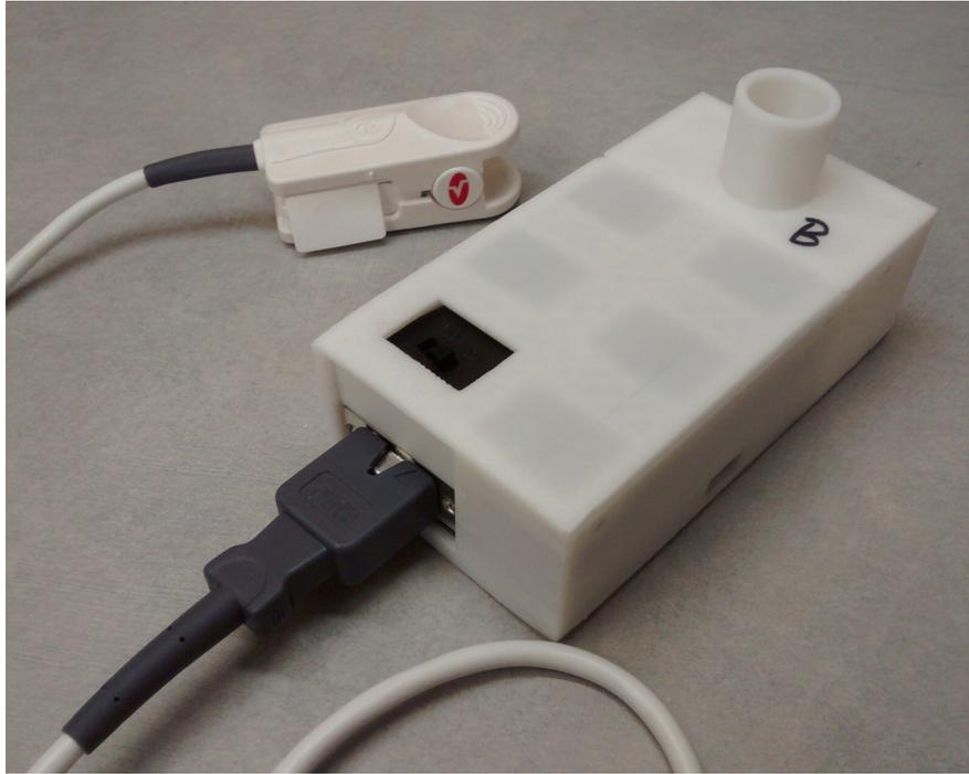
Figure 2.1: The sensor device with two components: (1) the finger-tip component on the upper-left and (2) the mouth component on the upper-right.
